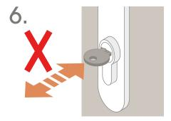
Do not use the thumb turn or key to pull the door open or closed.
