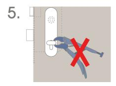
DO NOT FORCE the thumb turn with a device such as vice grips to increase leverage.
