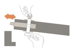
Figure 7 - Check the cylinder operates smoothly
