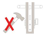
Figure 5 - Do not force the cylinder
