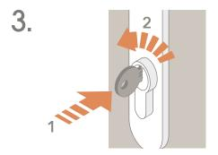
Make sure the key is inserted fully (1) into the cylinder before turning (2). DO NOT force the key to turn.
