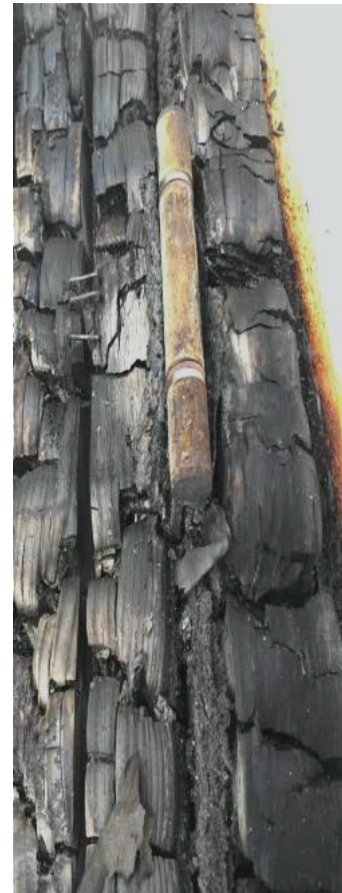
Graphite based intumescent seal once expanded
